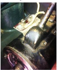
batteries. The best solution is to install a 'Fuse Mount Assembly', sold through the Snyders and Bratton's Catalogs. The assembly mounts directly to the side of the starter using the existing screws. Even the 'MAFCA Judging Standards' allows for this sensible addition. It will save your wires and stop the drain on your
